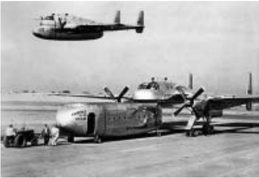
Figure 1. Fairchild XC-120 pack plane with detachable module. Courtesy of History Office, Air Force Aeronautical Systems Center.
